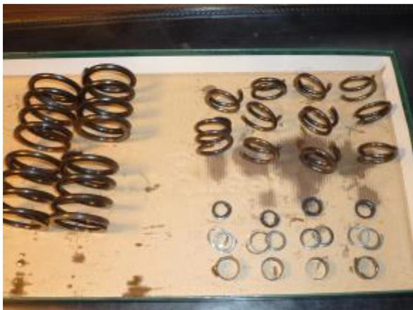
These broken springs damaged the valve guide seal caps and these thin metal fragments were what I had found in the oil filter cap during my service.
