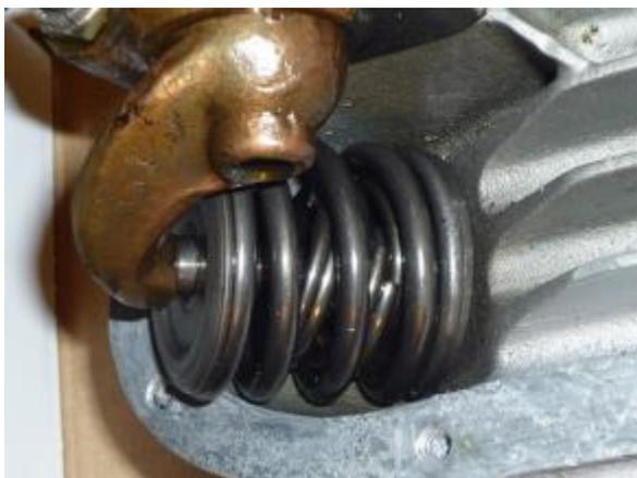
Why are the springs broken? They are over-hardened – bad quality (V-twin junk may be from China). Now I will install a valve spring set from the Kibblewhite Precision Machining USA. Finally: the oil filter saved the live of my motor. I had no metal fragments in the oil tank and no contamination in the oil feed line !
