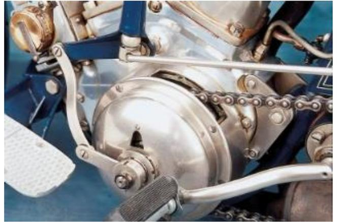
*The 1914 Thor was available in single and two-speed drive, the latter shown here with two speed drive.*
