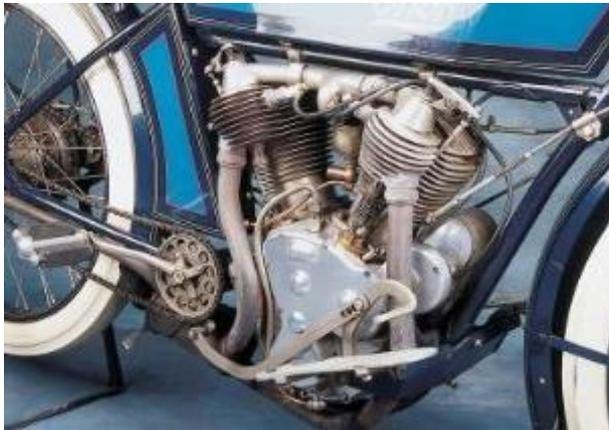
*The V-twin engine was of conventional intake-over-exhaust layout, but Thor ran the intake pushrods between the cylinder fins.*
