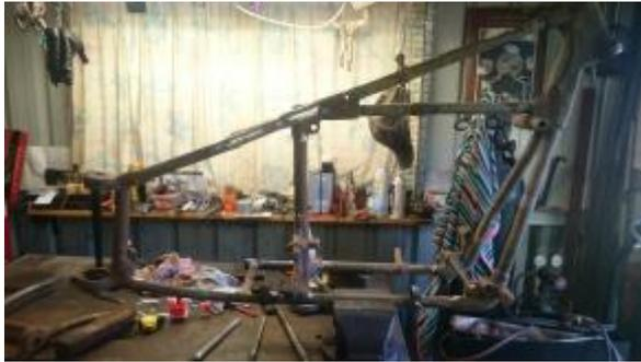
It took me about three days to get the centre section to almost perfect, and when I say almost perfect, I still have a half mm discrepancy in alignment. That is from the front wheel to the rear wheel through the frame. I'm still a half of a mil out, which is way better than factory and as good as most new bikes, so I was pretty happy.
