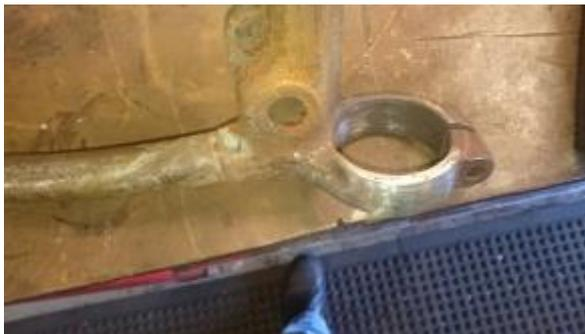
All up it took about a week to bring it back to almost perfect. So what's the result of all of that work? A very straight frame (straighter than factory), and a strong frame, because all of the welds have been redone or repaired.
