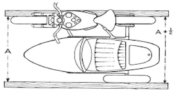
To ensure easy steering with a sidecar, the sidecar wheel should "toe-in" slightly towards the front wheel. The illustration shows how measurements should be taken between the wooden straight edges touching the wheels.
